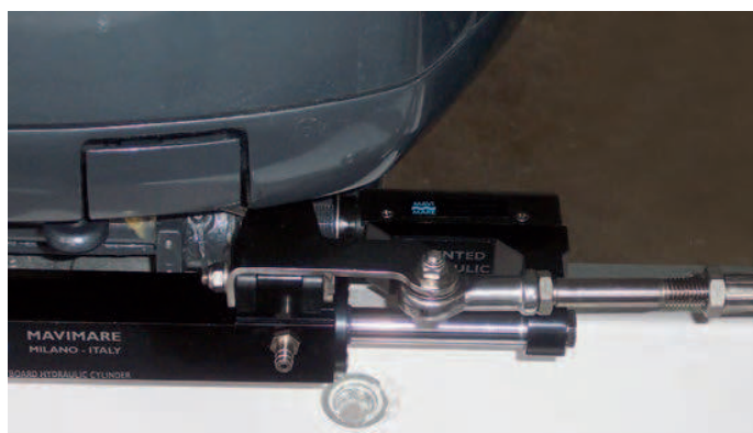
Installation of tie bar with art. X.345 - art. X.338
